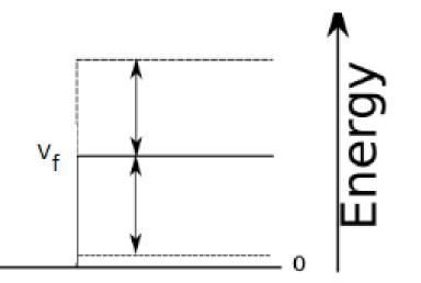
• A fermi potential can be modified in a  $V_{effective} = V_{Fermi} \pm \mu \cdot B$ magnetic field to only let one polarization through (see right)  $U = V_f^{iron} \pm |\mu_n| B_{sat} \sim 200 \pm 120 \, neV$   $B_{sat} \sim 2.7$
