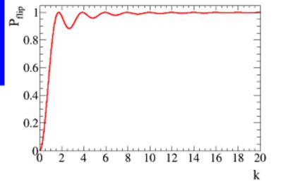
• For RF field following ~ sine function get an spin flip probability:  $P_{flip}=1-\frac{\sin^2(\pi\sqrt{1+k^2}/2)}{1+k^2}$ NIM Phys. Res. A 384(23) (1997) 451.
