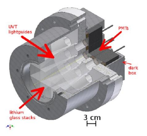
Made with aluminum (Al), a low density non-magnetic material
