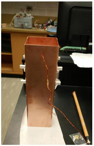
RF encased in copper shielding
