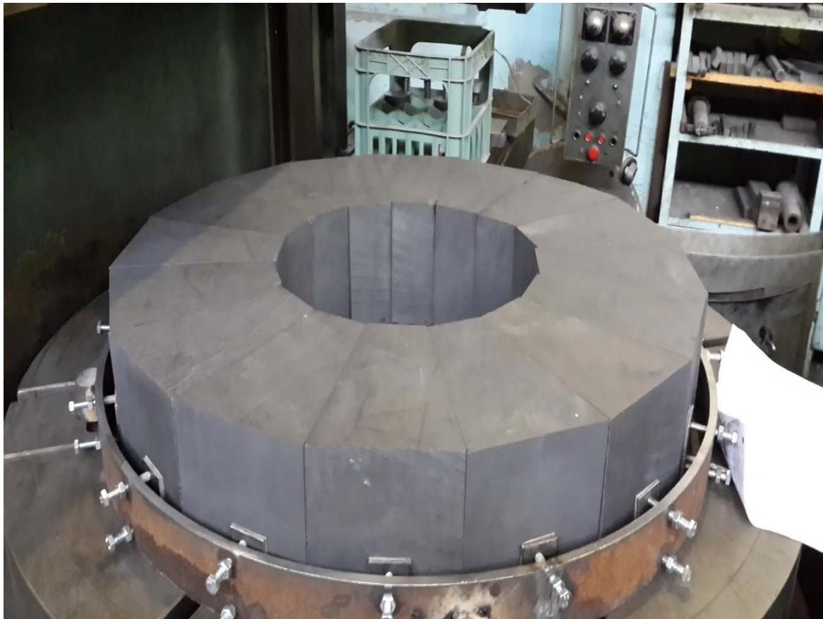
It is intended for the thermalization of neutrons and the creation of a  $4\pi$  irradiation geometry for the UCN source.
