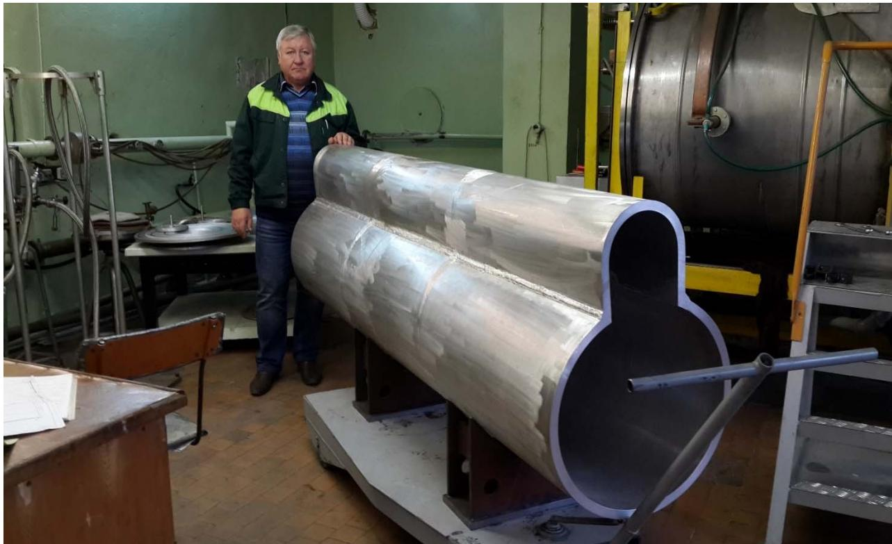
It is designed for reduction of heat inflows and localization of the beyond-design accident related to the explosion of hydrogen-air mixture inside the module.
