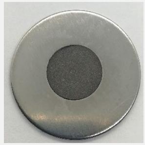
**Cr pellet:** Ø10 mm x 400 µm;  $\rho_{\text{Cr}} \sim 50\%$  bulk
