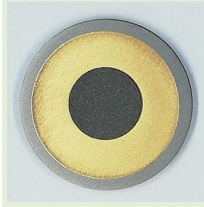
**Cr pellet:** Ø10 mm x 430 µm;  $\rho_{\text{Cr}} \sim 66\%$  bulk
