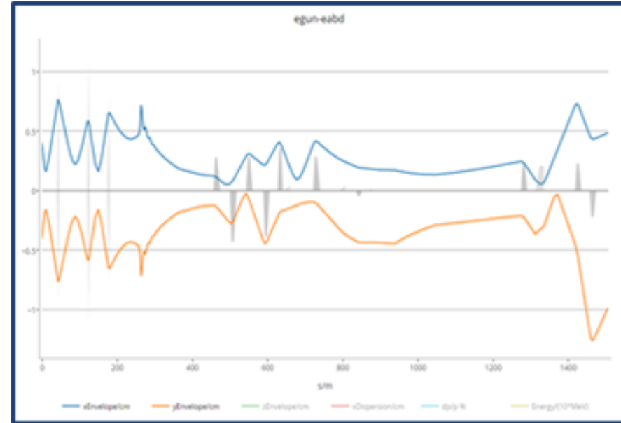
Beam envelope in e-linac calculated by TRANSOPTR (Rick Baartman)
