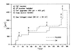
In the experiments with beam currents up to 420  $\mu A$  at 50% duty cycle, the dee was conditioned at  $\mathbb{H} \mathbb{K} V$ , and was set to 95 kV for operation. No system problems were encountered during this test. Beam loading had no substantial effect on the operation of the rf system. The instantaneous beam power was 210 kW with the resonator power approximately 1250 kW.
