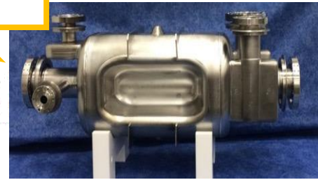
"CRAB" CAVITIES 16 superconducting "crab" cavities for each of the ATLAS and CMS experiments to tilt the beams before collisions.
