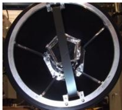
In-vacuum moving tape collector system
