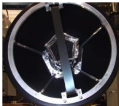
In-vacuum moving tape collector system
