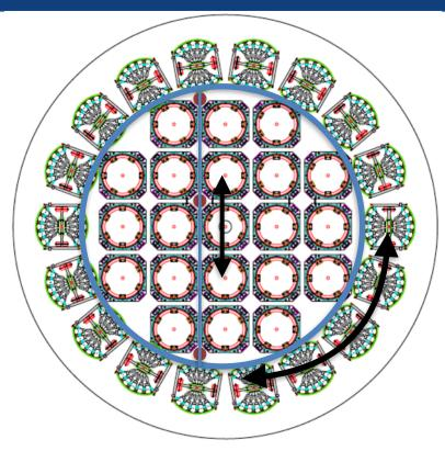
Use the same light source deployed at different positions (SNO calibration was in single plane)
