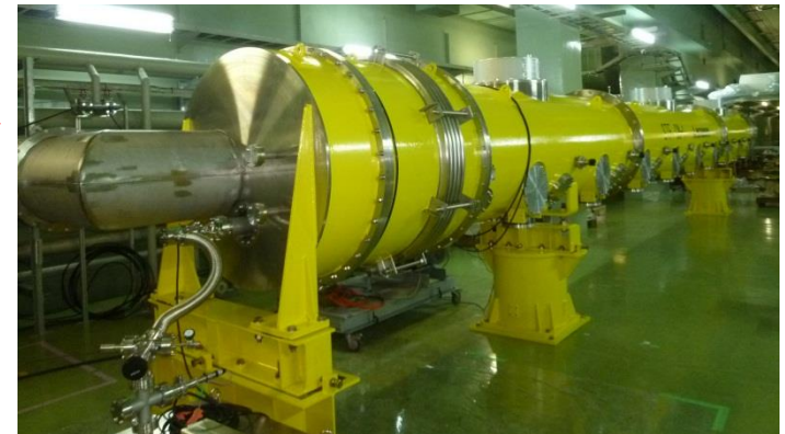
STF-2 - CM1+CM2a Cryomodule Eight + Four 9-cell cavities (2014')
