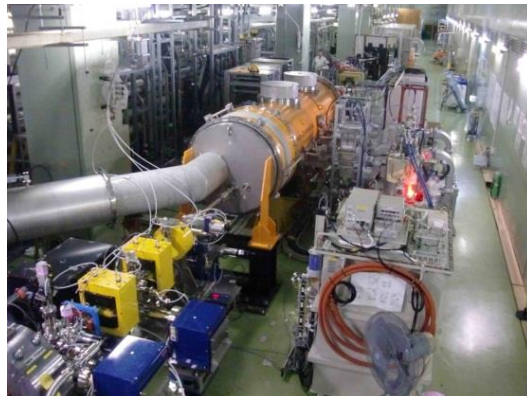
STF-2 - Capture Cryomodule Two 9-cell cavities (2012')
