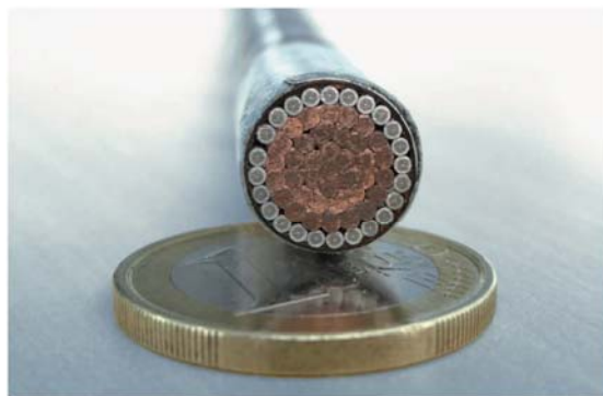
Photo of a superconducting cable composed of 24 MgB 2 wires and a copper core, and with a diameter of only 11 mm. Such cables can carry currents of 10 kA and more.
