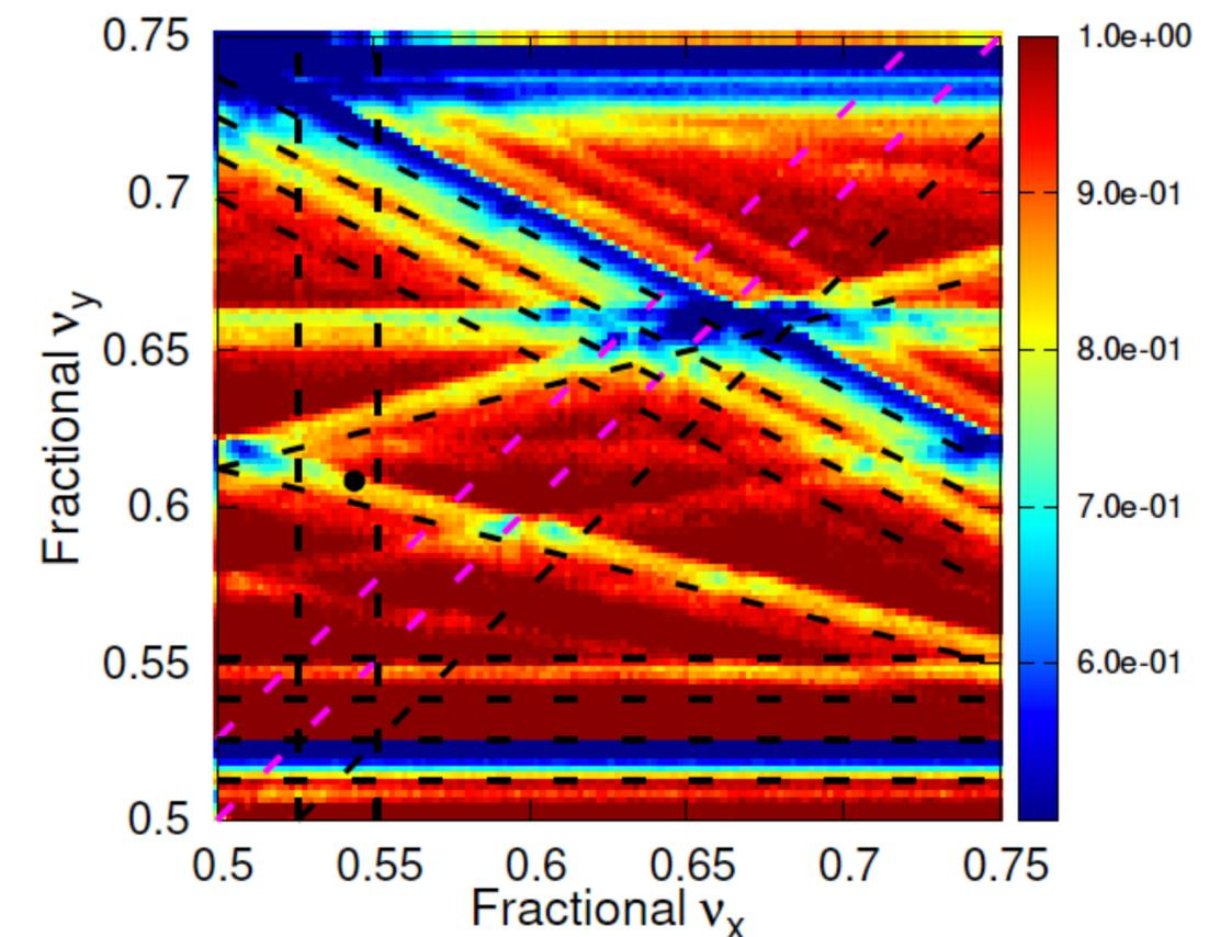
Luminosity tune scan: BBWS simulations with weak e- beam using parameter set of 2019.04.02
