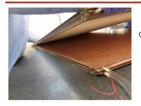
one doublet lowered over another doublet while pushing against the alignment pins
