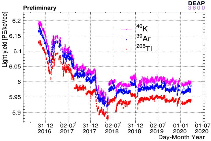
Light yield values of detector was calibrated by fitting the <sup>39</sup>Ar, <sup>208</sup>Tl and <sup>40</sup>K peaks
