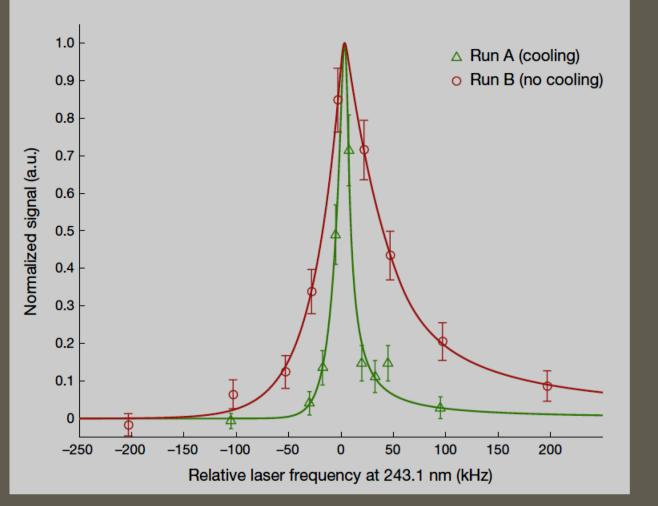
A set of laser cooled 243nm spectroscopy runs were performed using the same experimental procedure as the 121nm runs
