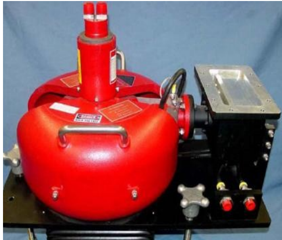
2001 - 2011 8kW klystron VKL7811St from CPI
