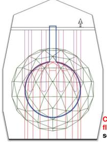
Jongen et al. 1993, IBA Industrial 10 MeV 20 mA Rhodotron diameter 2.9 m, 49% efficiency, 108 MHz, few M\$
