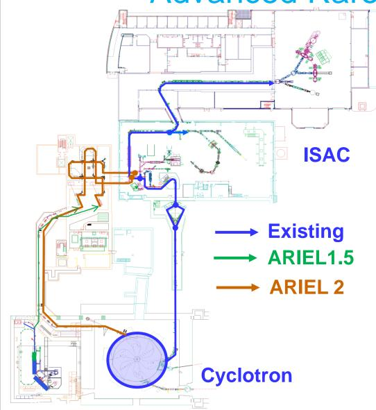
ARIEL will triple the lab's RIB production by adding two new target stations resulting in up to three simultaneous ion beams
