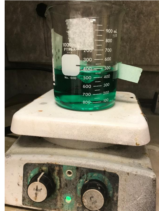
NiP plating solution on stir/hot plate
