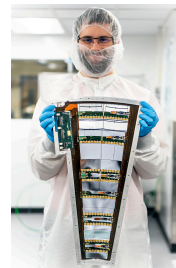
Fig: Tyman from the TRIUMF ATLAS group, holding an ITk detector segment.
