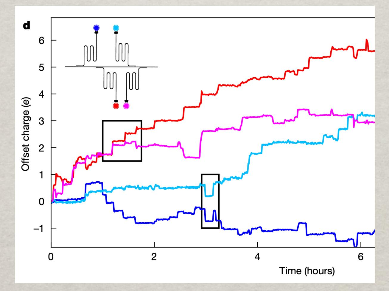
Measuring offset charge over long times Correlated noise also appears Correlated noise breaks most quantum-error correction
