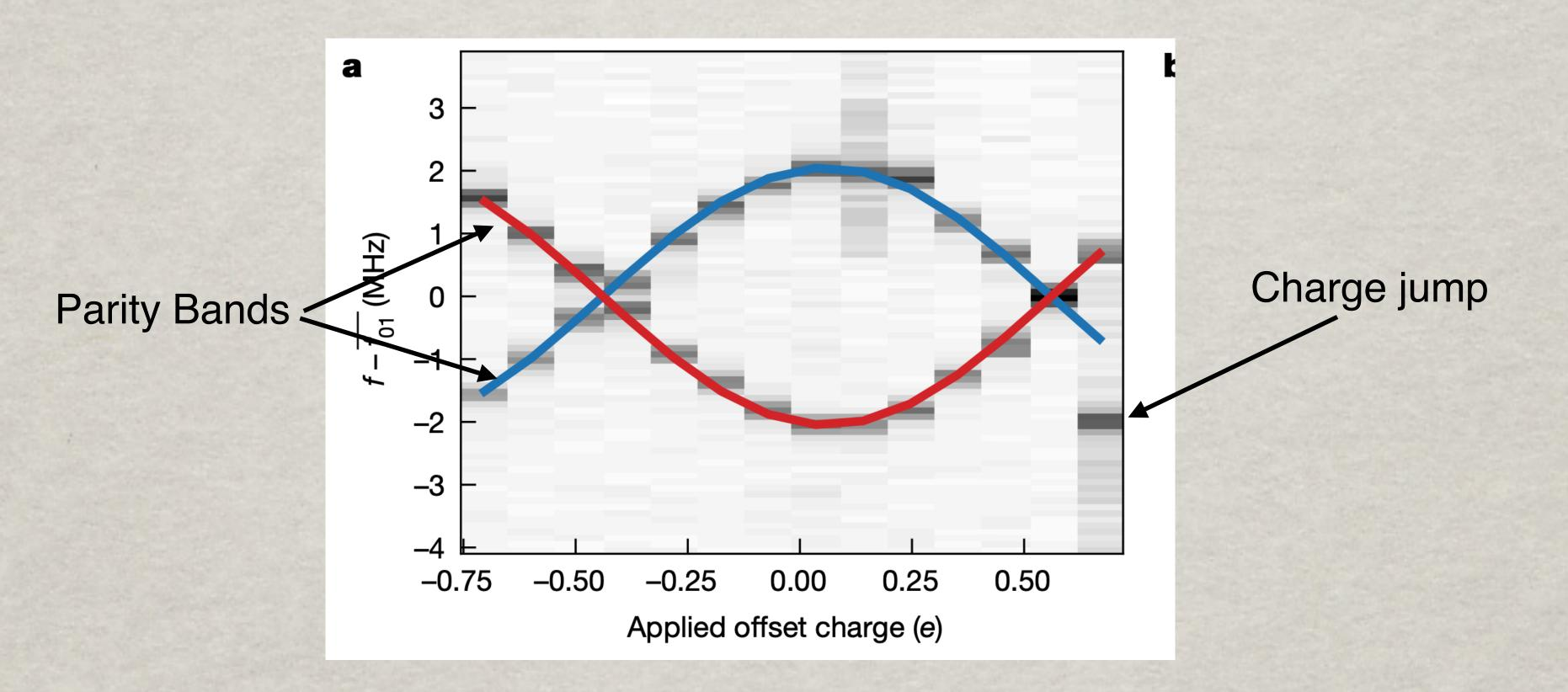
Red and blue bands reflect switching of QP parity Discrete charge jumps also observed (on right edge)
