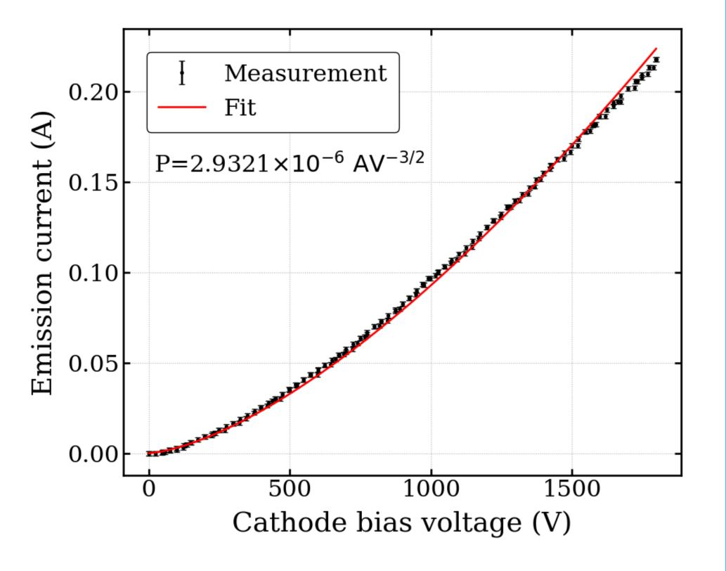
The TITAN EBIT perveance is about 2.9e-6 A V<sup>(-3/2)</sup> or 2.9 µPerv. Above 1500 V there is a small deviation from the space-charge limited emission indicating an underheated cathode.
