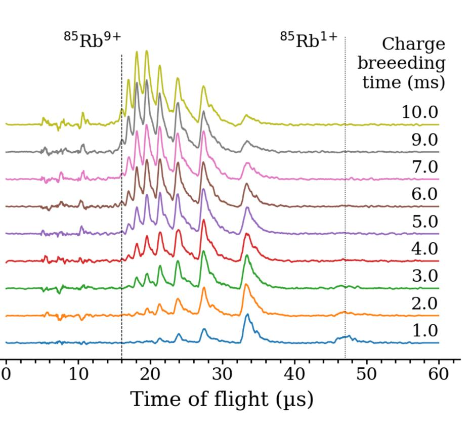
HCI spectrum for the same electron current (100 mA). By increasing the breeding time, higher charge states are populated. In this case, <sup>85</sup>Rb<sup>9+</sup> is achieved as of 5 ms.
