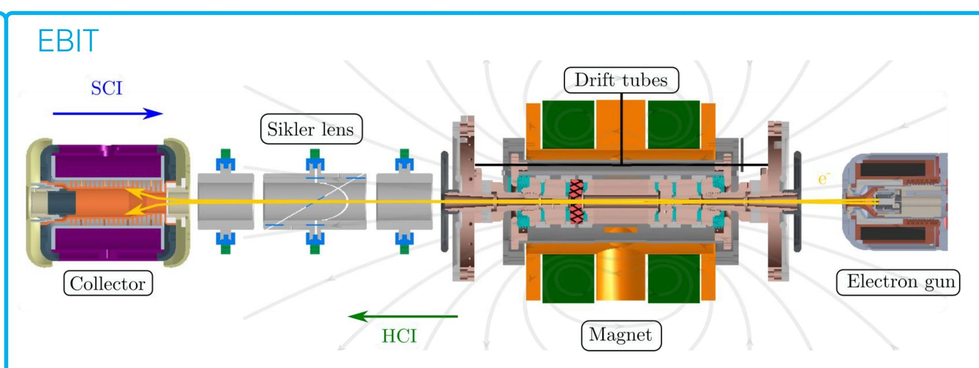
The EBIT consists of an electron gun, a set of electrostatics drift tubes, a semi-Helmholtz coil, and an electron collector. HCIs are created by successive electron impact ionization from the SCI injected into the drift tube region (red, cross-hatch). EBIT design for 5A, 60 kV, and 6T.
