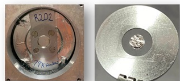
Ultra-Thin (120 nm) Thermal windows
