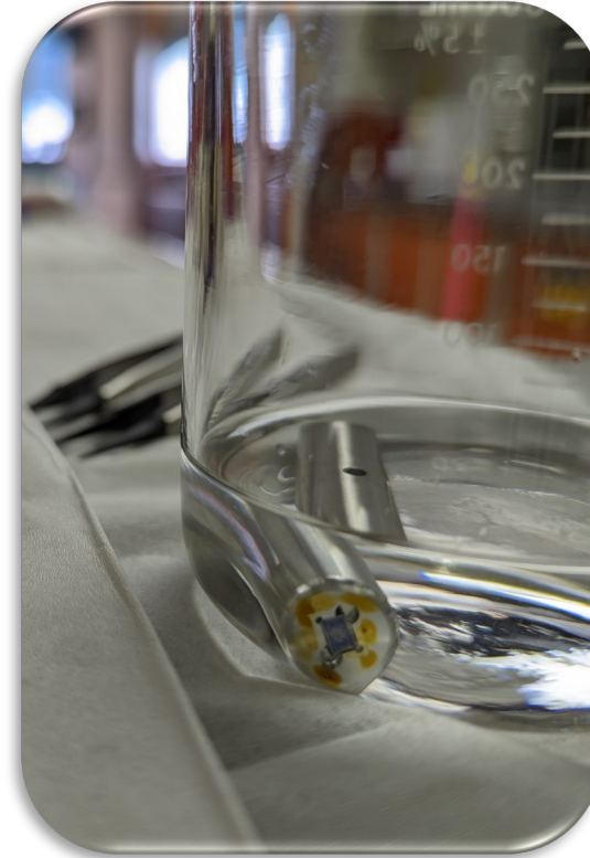
Holder + STJ array in ethanol bath
