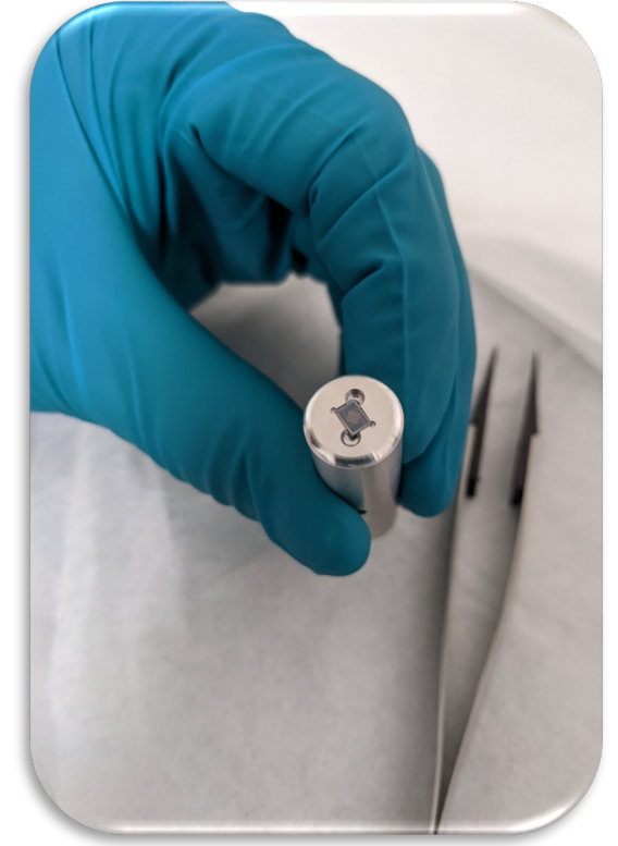
STJ array without Si collimator (removal after ethanol rinse with carbon-tip tweezers)
