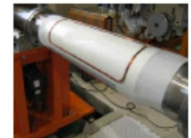
TiN-coated beam pipe with antechambers
