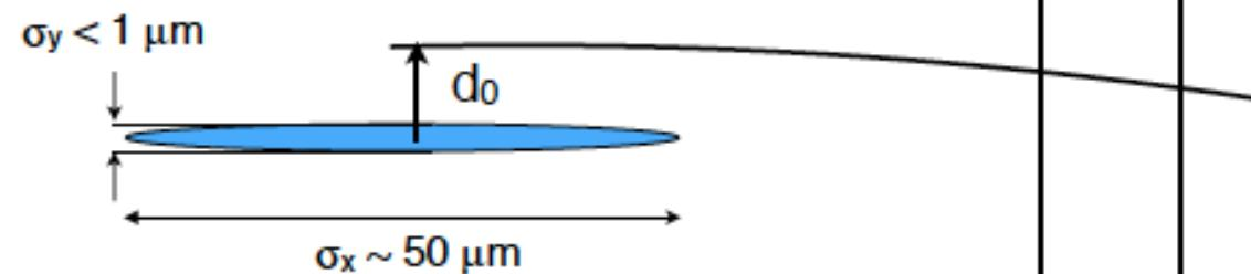
Transverse impact parameter,  $d_0$ , resolution is **12 μm (CDC+SVD+PXD)** (expected is 10 μm).
