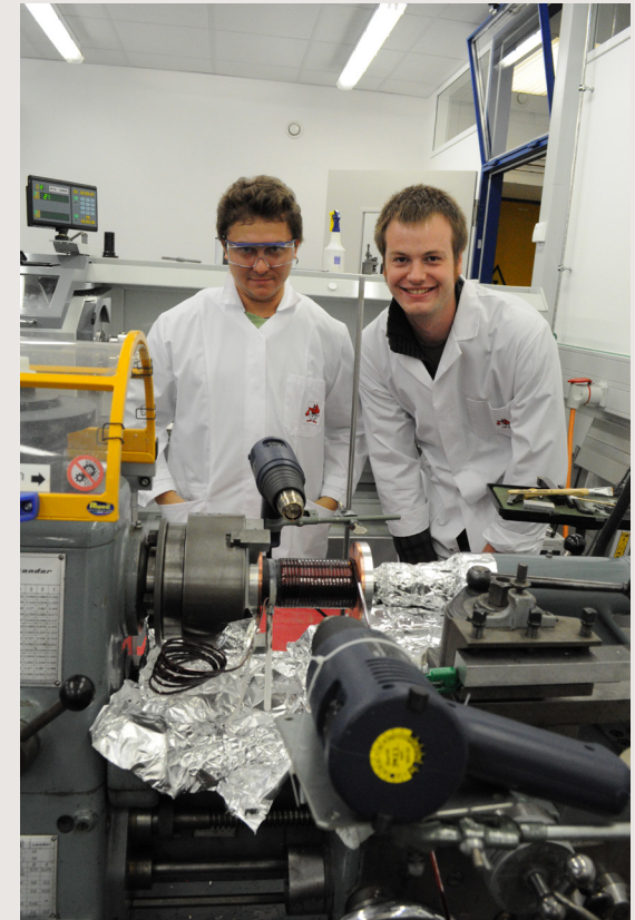
The magnetic coils for electron gun and collector needed to be wound and glued manually
