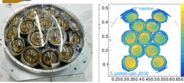
Successful optical and hydrostatic pressure tests of the prototype multi-PMT photo detection modules built at TRIUMF
