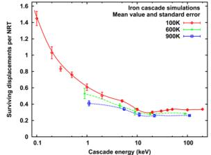
**Temperature dependence.** The calculations of Stoller (J. Nucl.Mater. 276 (2000) 22) for iron at 100-900K show some temperature dependence of the number of stable defects. At the same time the comparison of displacement cross-sections for p+Fe calculated using Stoller defect generation efficiency with the displacement cross-sections derived by Jung (J. Nucl. Mater. 117 (1983) 70) from low temperature experiments shows very good agreement.
