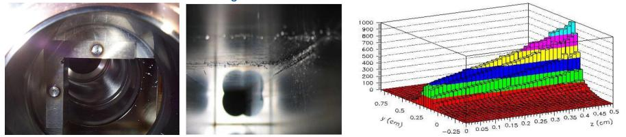
Detailed modeling of dynamics of beam loss (STRUCT), energy deposition (MARS15) as high as 1 kJ/g, and time evolution over 1.6 ms of the tungsten collimator ablation, fully explained what happened
