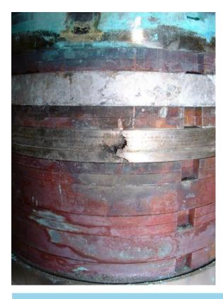
FNAL pbar production target under 120-GeV pbeam (3e12 ppp,  $\sigma \sim 0.2$  mm)
