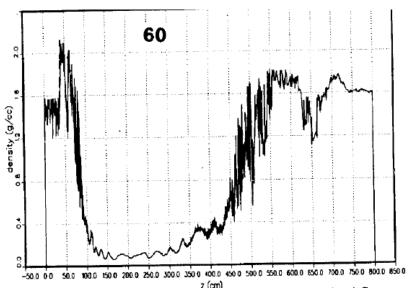
The hole was drilled at the 7 cm/ $\mu$ s penetration rate. Shown is axial density of graphite beam dump in 60  $\mu$ s after the spill start
