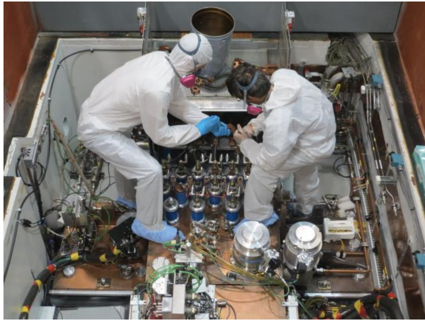
Connecting a Target Module in the pit
