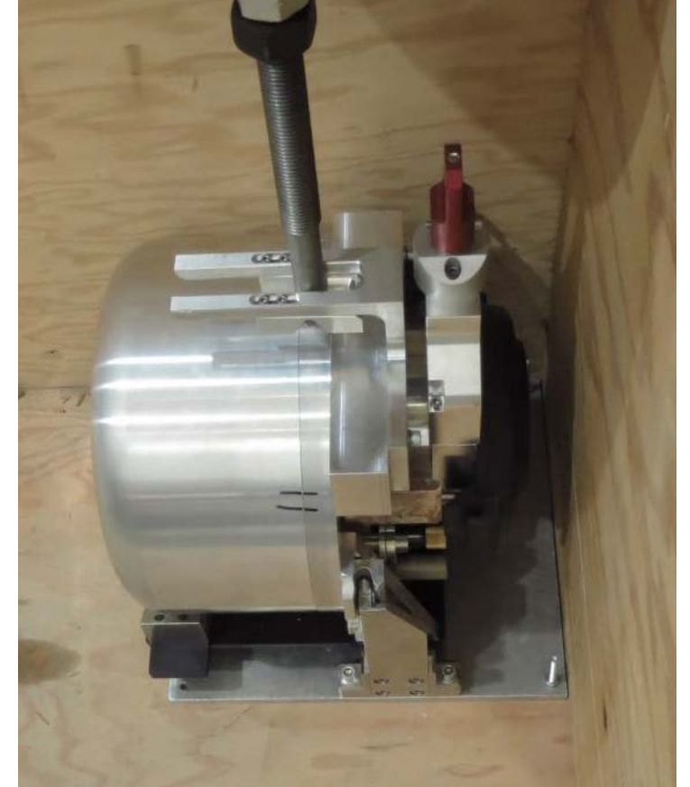
Successful local pick-and-place of ISOLDE target vessel (much closer to ARIEL design) object via Remote Handling crane onto ISOLDE locating pin design – 16-March-2018
