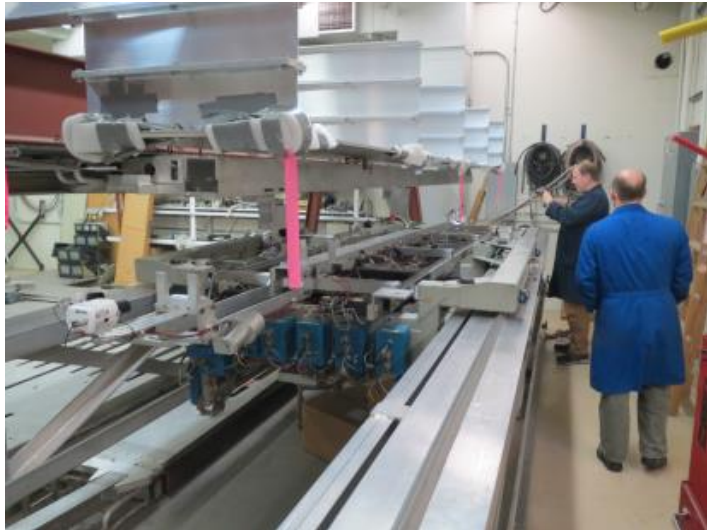
Off-line mockup test of cyclotron trolley (HE probe service)
