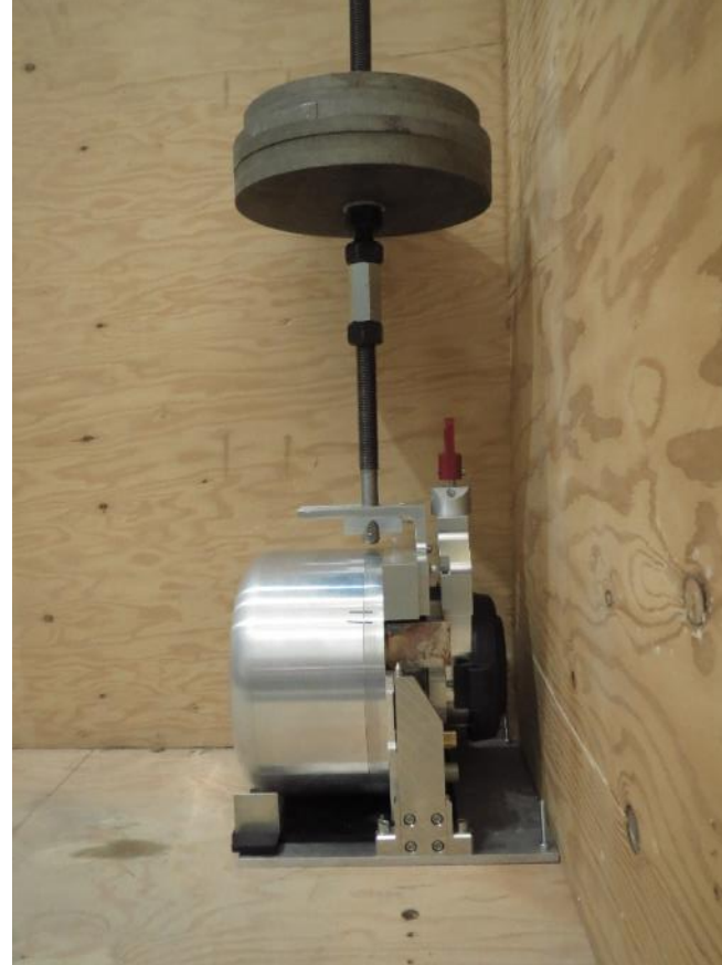
Successful local pick-and-place of ISOLDE target vessel (much closer to ARIEL design) object via Remote Handling crane onto ISOLDE locating pin design – 16-March-2018
